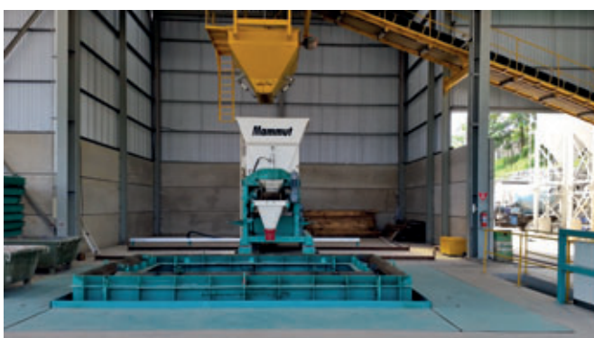
Mammoth 8668 - the largest vibrating table that BFS has ever built
