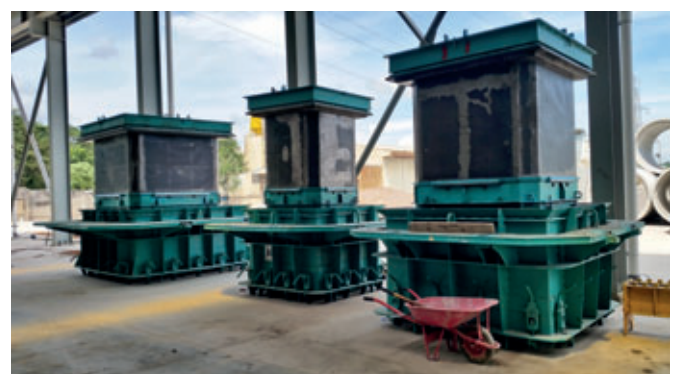
Box culvert moulds for the Jumbo for different product sizes
