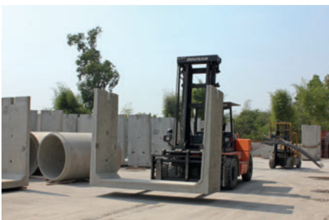
A U-ditch being loaded.
