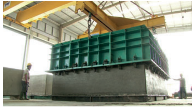
A box culvert manufactured on the Mammut vibrating table pictured during demoulding
