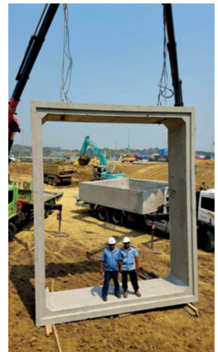
The name says it all: large box culverts can be manufactured on the Mammut plant
