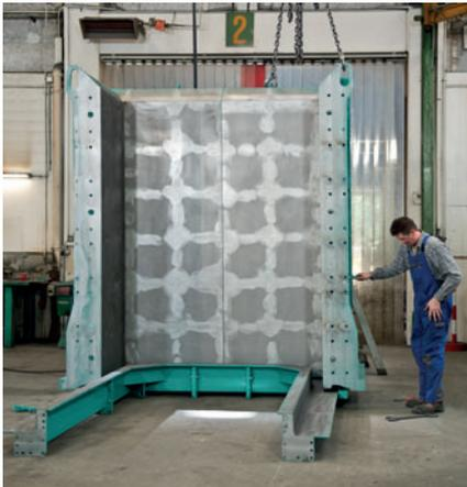
Assembly of precisely shaped modular mould parts.
