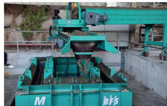
*Mammut production with rotating discharge belt and CNC path control.*
