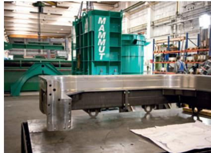
Finitec spigot-end mould for precise, clean joints
